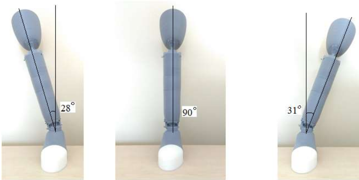
Figure 8. The front view of the prosthesis. Eversion, upright posture, and inversion movements.
