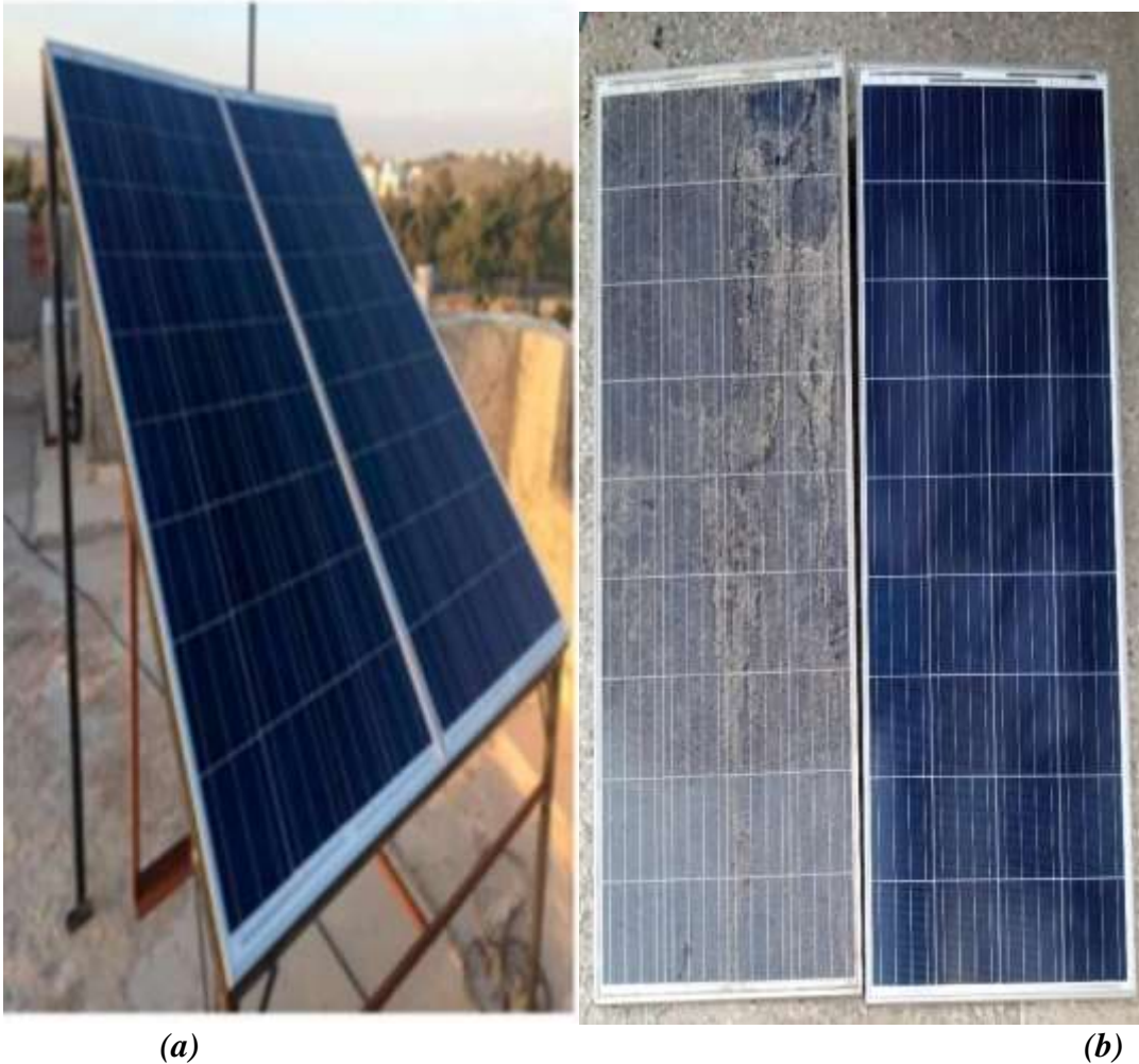
Fig 2: Real Picture of the considered PV system: (a) Reference case (b) Dust module
