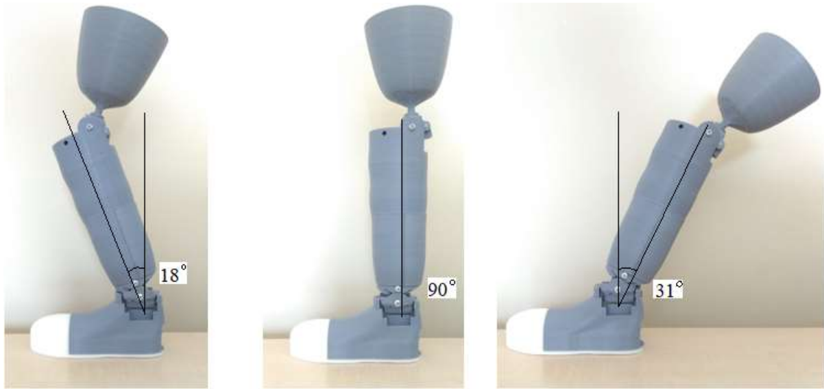
Figure 7. The sagittal plane view of the prosthesis. Dorsal flexion, upright posture, and plantar flexion movements, respectively.
